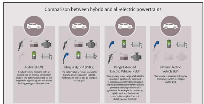
Fig. 1. Comparison of electric and hybrid drive
