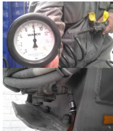
Fig. 5 Pressure on the control line at the coupling.
