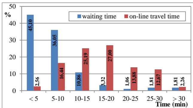
Fig. 1. Passenger waiting and on-line travel time
