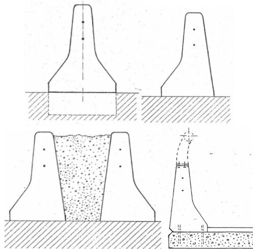
Figure 2. Classification of protective concrete bunkers (New Jersey)
