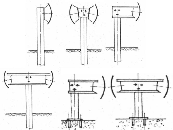
Figure 1. Classifications of steel guardrails
